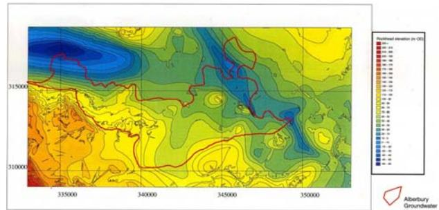
Figure 10. Elevation of the Bedrock surface around Shrewsbury (located centre right); blue is below present-day sea level. Taken from Bridge *et al.* (2001) and reproduced with permission of the BGS. (IPR/81-33c British Geological Survey © NERC 2008)
