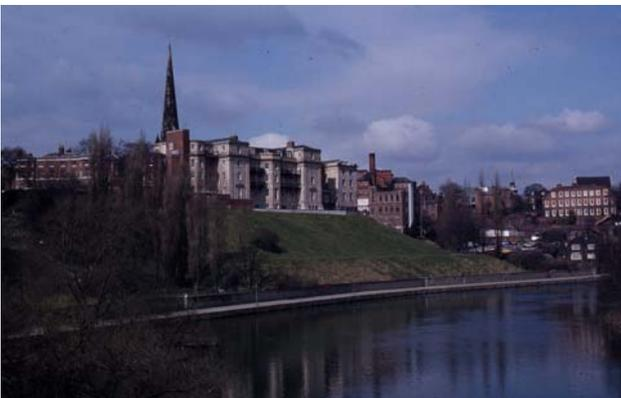
Figure 13. The location of a substantial landslide on the north bank of the Sever in central Shrewsbury, induced by high groundwater pressure caused by flow through the sand of a buried channel. © Copyright 2007 David Pannett
